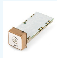
LS20126 receiver. Has a very small antenna, but works decently in open areas.
