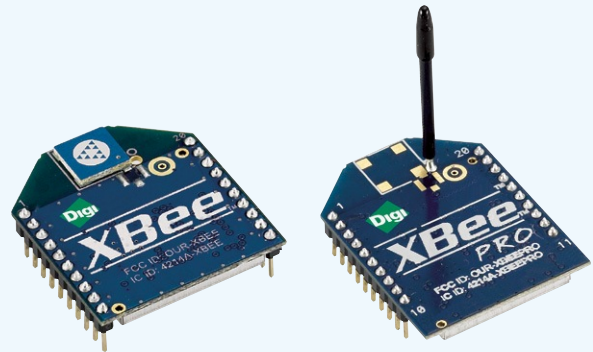
Figure 6-9. XBee 802.15.4 modules. XBee low-power module with chip antenna on the left, and XBee-PRO extended range module with wire antenna on the right.
