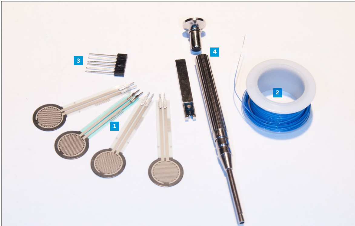
Figure 3-1. New parts for this chapter: 1. Interlink Series 402 force-sensing resistors (FSRs) 2. 30AWG wire-wrapping wire 3. Wire-wrapping pins (or long female headers) 4. New tool: wire-wrapping tool. The wire stripper to the left of the tool lives inside the handle. Don't forget plenty of male header pins for the breakout boards.
