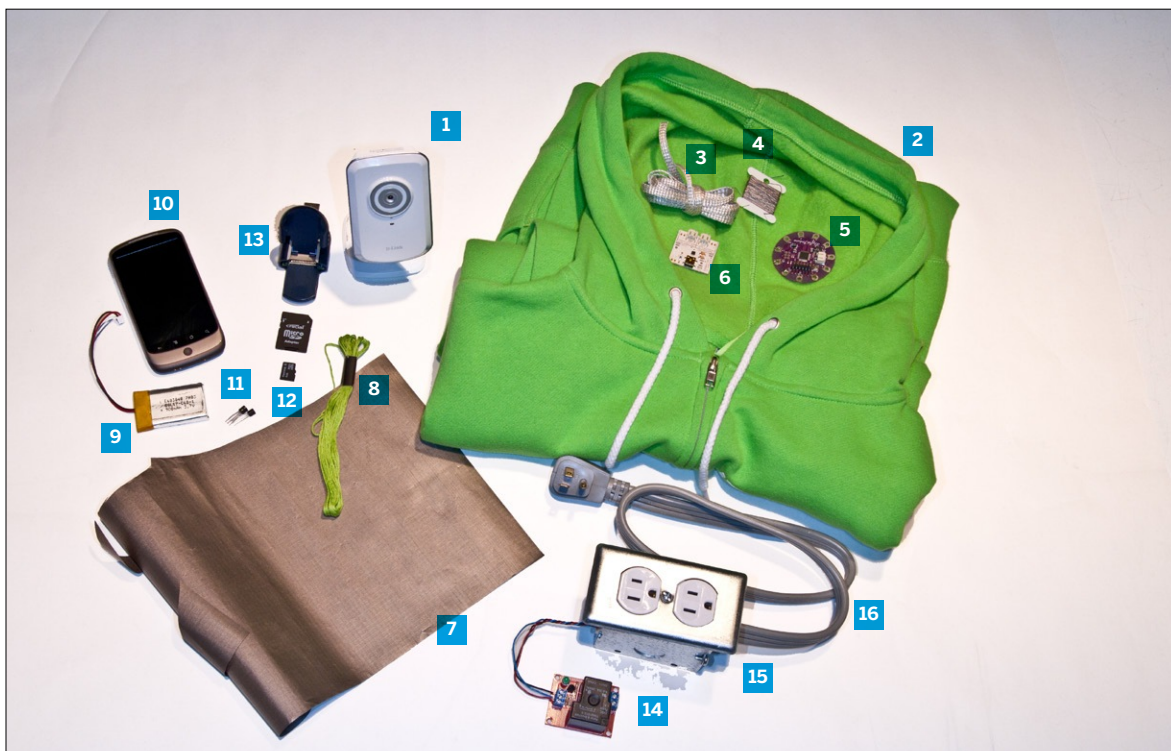
Figure 10-1. New parts for this chapter: 1. IP-based camera 2. Hoodie 3. Conductive ribbon 4. Conductive thread 5. LilyPad Arduino Simple 6. Lithium Polymer battery charger 7. Shieldex conductive fabric 8. Embroidery thread 9. Lithium Polymer battery 10. Android device 11. TMP36 temperature sensors 12. MicroSD card 13. MicroSD card reader 14. Relay board 15. AC junction box and socket 16. AC cord.
