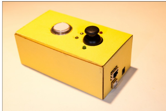
Figure 5-7 The assembled joystick controller. The joystick circuit inside the housing was designed to be just tall enough so that the LEDs and joystick would stick through the top. Assemble the circuit first so you know how much space you need for the housing. A cable made from scrap stranded wire and male headers to connect the pushbutton makes it easier to open and close the box with the button mounted. The inner wires from a telephone cable work nicely for this.
