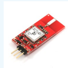
GPS MiniMod with GR10/MN1010 receiver. Smallest I could find. Takes a long time to acquire a signal.
