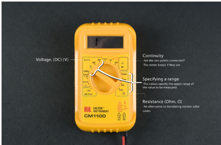
Figure 1-26. The most common functions of a multimeter
