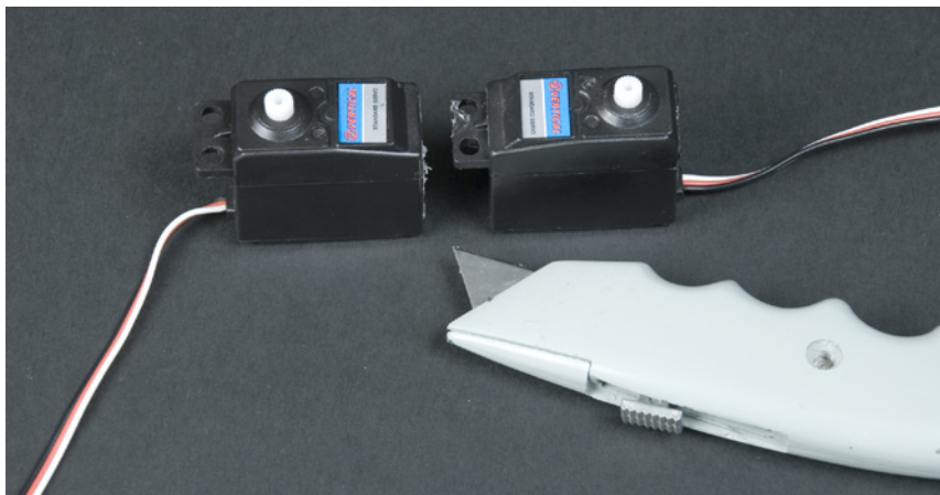
Figure 4-12. Removing the obstructing plastic
