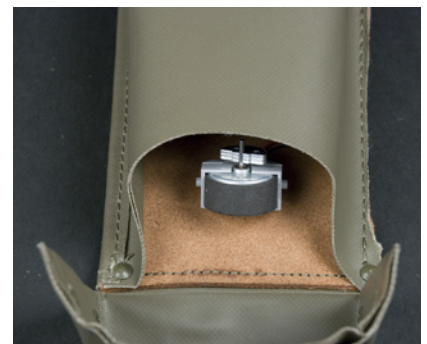
Figure 3-25. The vibration motor in place
