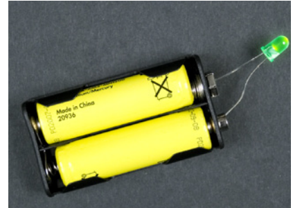
Figure 1-28. Simple closed circuit powering an LED
