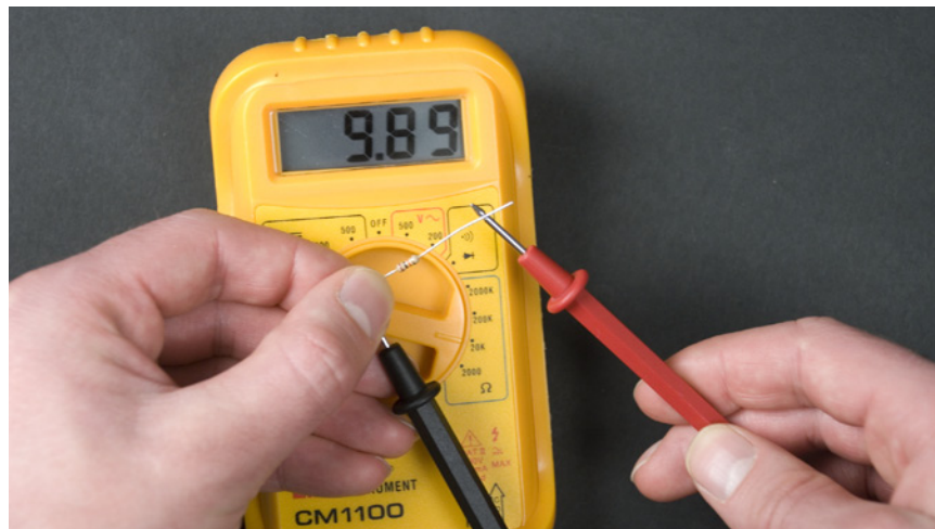
Figure 5-6. Measuring resistance with a multimeter
