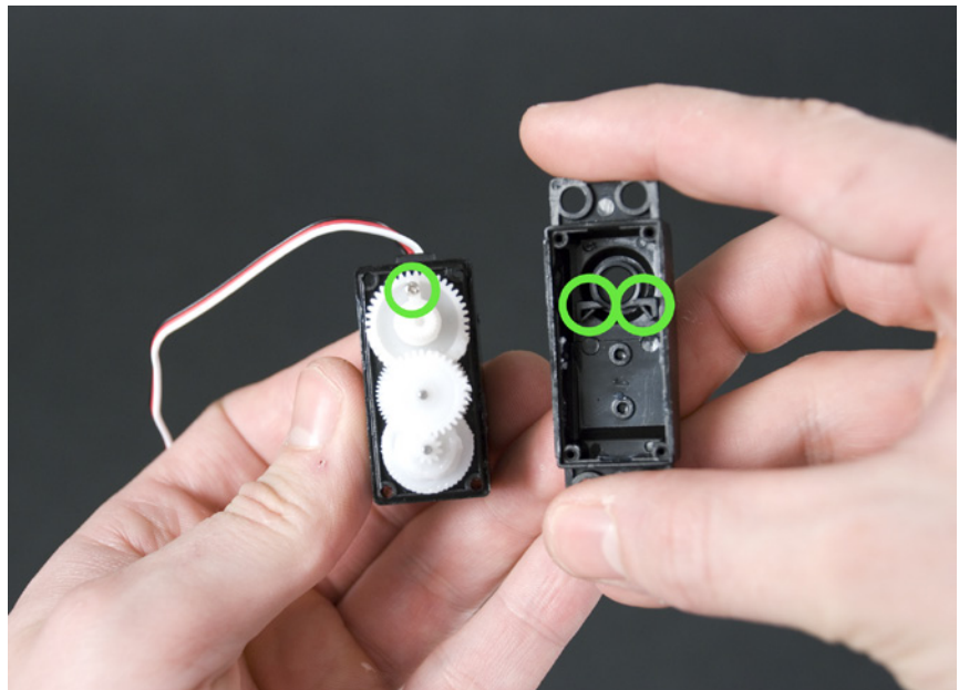
Figure 8-9. Obstructions that block rotation
