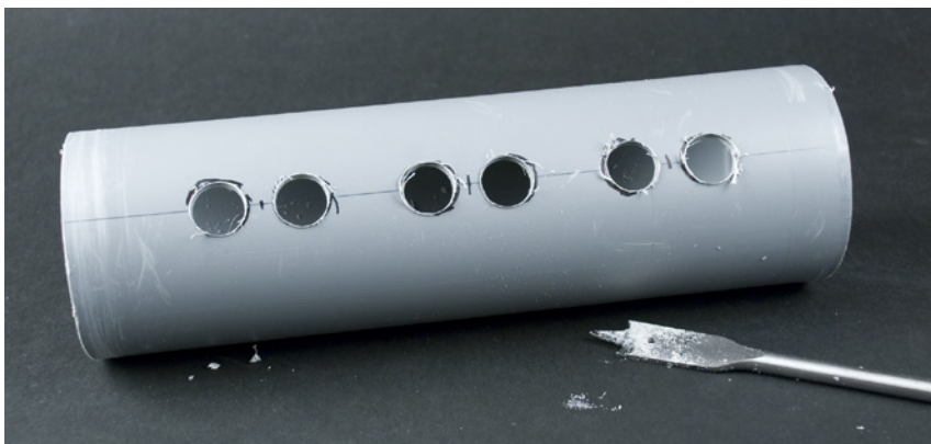
Figure 5-29. The 16mm holes for the sensors
