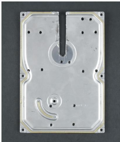
Figure 8-30. Drilled 3mm holes and notch cut for the kicker leg
