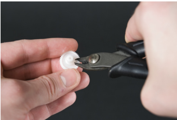
Figure 8-10. Cutting off the obstructions
