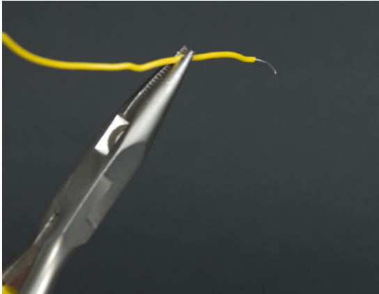
Figure 4-21. Bending the wire
