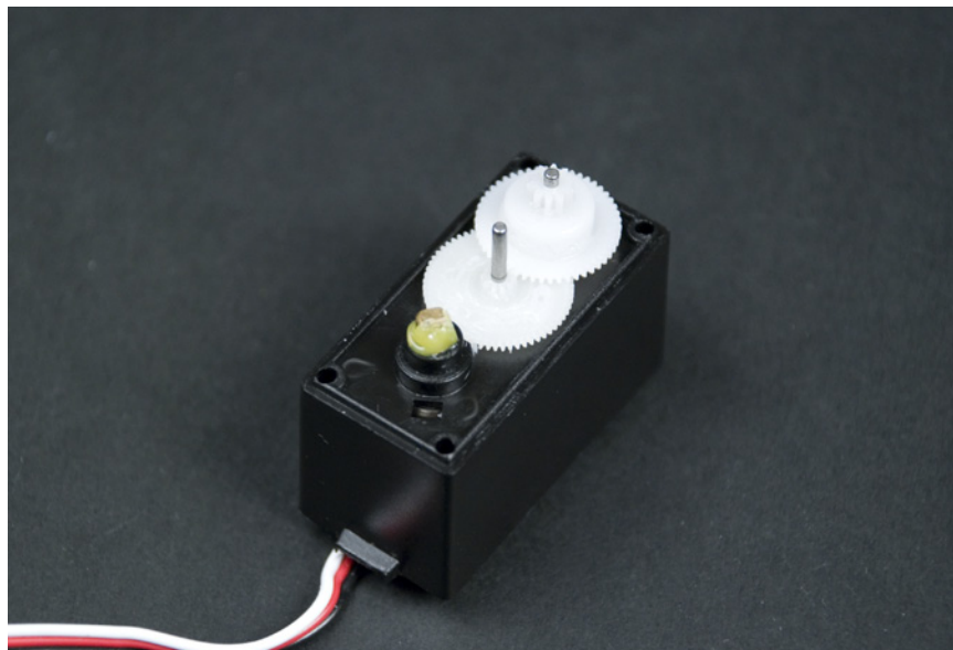
Figure 8-16. Using a drop of hot glue to hold the shaft of the potentiometer in place
