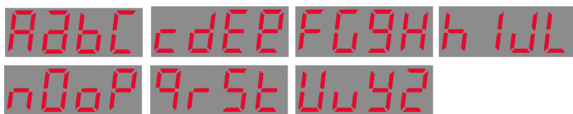
Figure 3-2. How English letters look on the seven-segment, four-character display.
